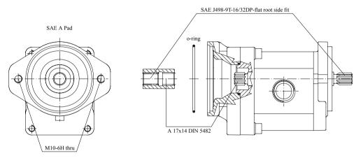
Dimensions for SNP2NN / 06SL flange/shaft option with auxiliary mounting pad kit installed
